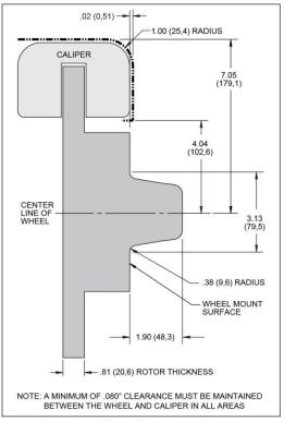
Figure 2. Wheel Clearance Diagram
