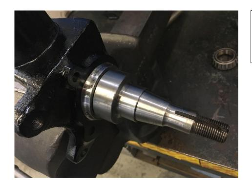
Once the bearing adaptors have been heated, install them on to the stub axles, making sure they have been fitted correctly
