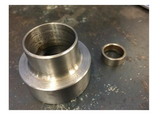
Bearing adaptor and bearing extension sleeve
