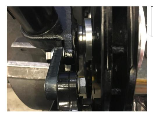
This photo shows the Caliper bolted to the Bracket and Stub axle using the spacers shown above
