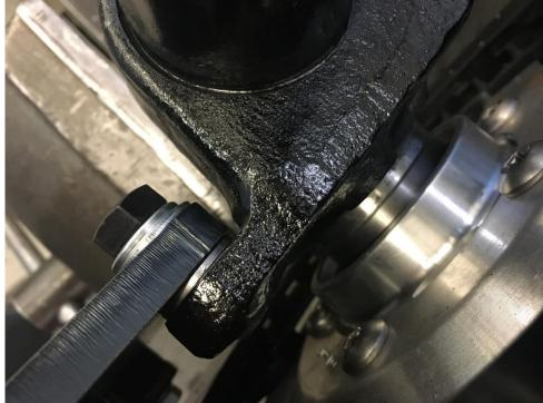
The Spacer will need to be fitted to the stub axle side then the caliper bracket and bolted using the Supplied bolts flat & spring washers
