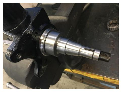
The bearing extension sleeves can now be fitted to the stub axles
