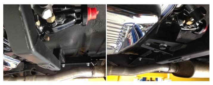
The fitting of the rear shocker mounting bracket is done using the same procedure. Use original shocker mounting holes as a guide to line up new unit.
