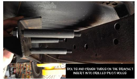
Tig weld these tubes to the chassis on both sides (Welding tubes is optional). Use supplied bolts, nuts and washers.
