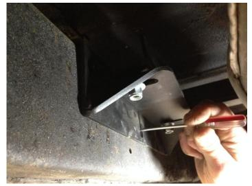
Remove transmission, drill 1/4" pilot holes. Use right angle drill if experiencing difficulty with clearance.
