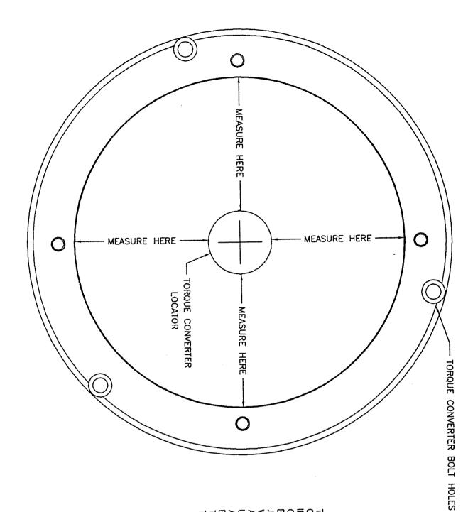
TO SET ALUMINIUM DRIVE RING TRUE TO TORQUE CONVERTER LOCATOR, CAREFULLY FOLLOW THESE INSTRUCTIONS \* BOLT THE RING TO THE TORQUE CONVERTER, REFER TOP INSTRUCTION No. 6.
